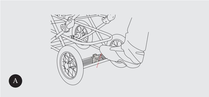
Clean the brake regularly, rinse it off and lubricate it, in order to maintain an effective brake function. We recommend that sewing machine oil is used.
